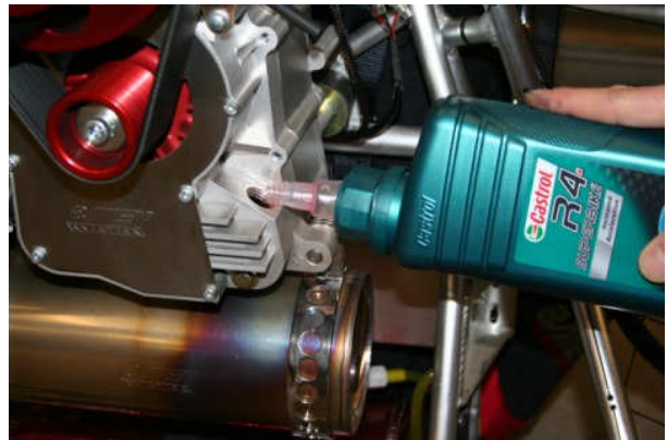
Oil filling location
