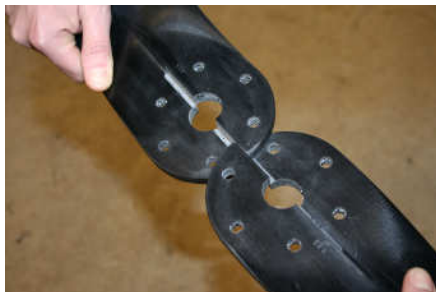
Propeller halves slide together
