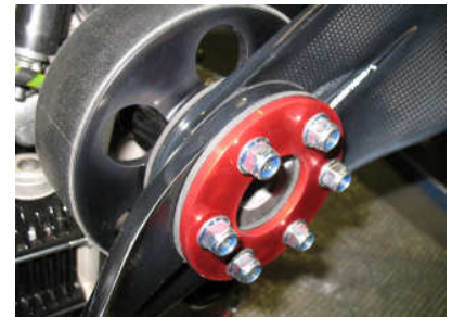
Engines after February 2008 Two rubber gaskets Secured with 6 x M8 Nuts
